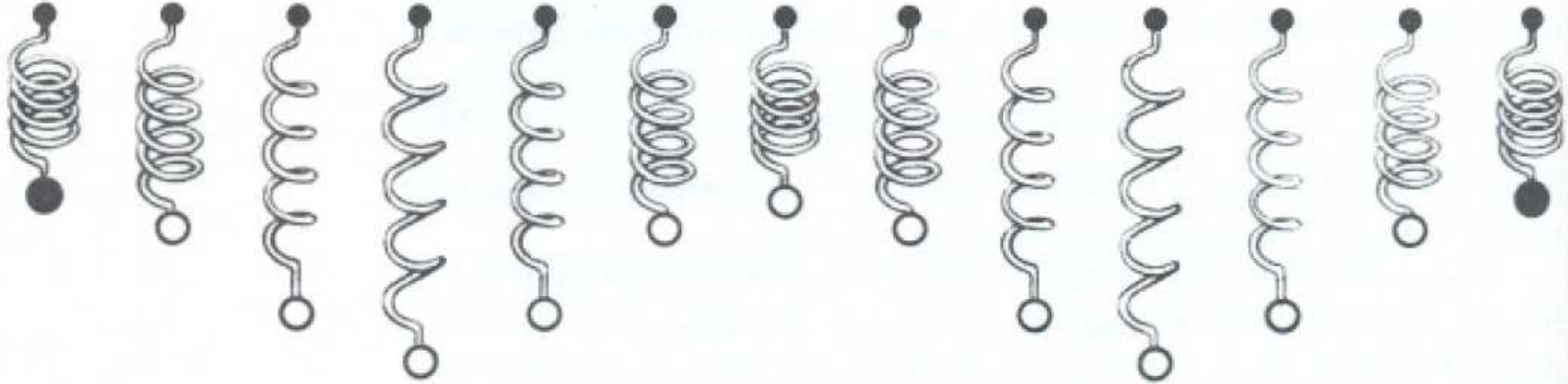
FIGURE 4-3 Synthesis of a wave from an assembly of independent oscillators.
