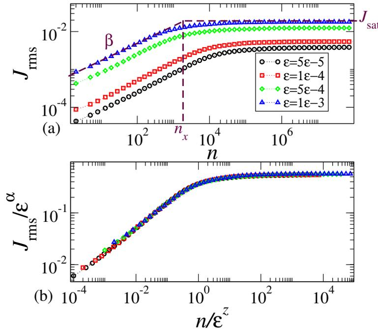
**Fig. 1** Plot of: (a)  $J_{rms}$  vs.  $n$  for different values of  $\varepsilon$  and considering  $\tilde{f} = \cos(\theta)$  in mapping (1). (b) After a properly rescale in the axis, all curves overlapped onto each other in a single and hence universal curve. The parameters used were  $\gamma = 1$  and  $M = 1000$  different initial conditions chosen as  $J_0 = 10^{-3}\varepsilon$  and  $\theta_0 \in [0, 2\pi]$ .
