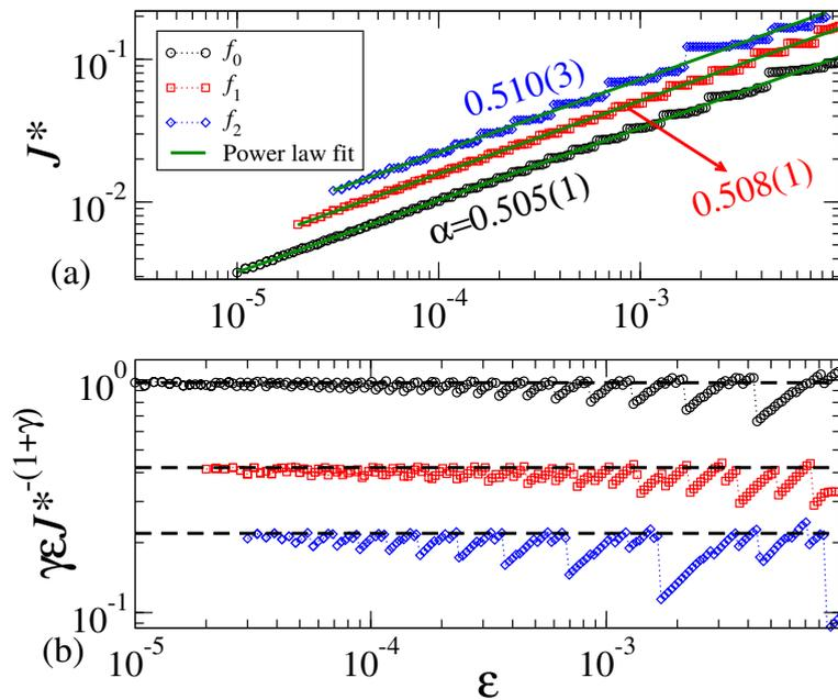
**Fig. 5** Plot of: (a) Approximated position for the minimum of the lowest invariant spanning curve ( $J^*$ ) as function of the control parameter  $\varepsilon$ . The orbits were iterated up to  $10^{11}$ , and we have considered  $J_0 = \theta_0 = 10^{-6}$  and  $\gamma = 1$ . (b) Rescale in the vertical axis of item (a)  $J^* \rightarrow \gamma \varepsilon J^{*-(1+\gamma)}$ , where the dashed lines are the values of  $K_c(f_i)$  found numerically for the generalized standard mapping.
