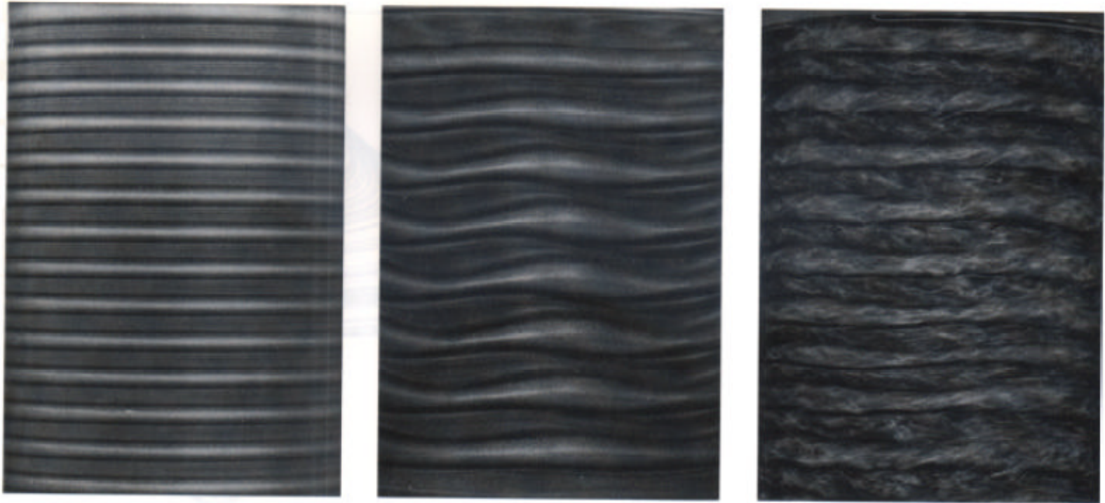
FIGURE 1. Patterns formed in water contained between concentric cylinders with the inner cylinder rotating: a steady pattern of stacked donut-shaped rolls. b waves on the rolls. c chaotic flow. The patterns are made visible by adding a small amount of flat flakes (often ground up fish scales) that align with the flow.
