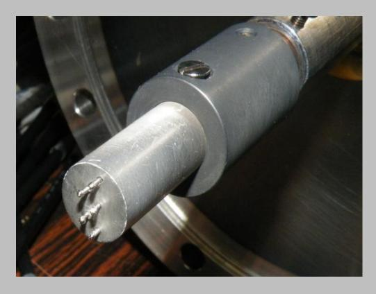
The probes were installed in the equatorial plane of TCABR. Each probe has a movable system that allows to put it in different radial positions (shot by shot) in a range of [+2.0 to -3.0] cm, or  $r/a \approx [0.9, 1.2]$ , with respect to the limiter.
