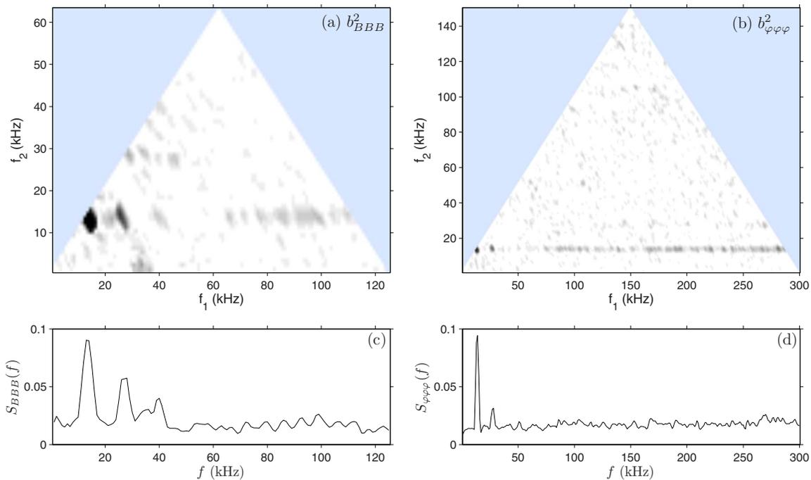
FIG. 3. (Color online) Bicoherence spectrum of (a) magnetic ( $b_{BBB}^2$ ) and (b) electrostatic ( $b_{\varphi\varphi\varphi}^2$ ) oscillations during high MHD activity (between 40 and 60 ms). (c) and (d) are plots of the summed bicoherence corresponding to (a) and (b), respectively.
