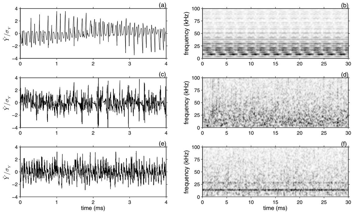
FIG. 5. Time evolution of the normalized electrostatic oscillation amplitude obtained from numerical integration of Eqs. (10)–(12) with (a)  $A=B=0$ ; (c)  $A=0.35$ ,  $B=0$ ; (e)  $A=0.35$ ,  $B=0.03$ . The spectrograms in (b), (d), and (f) correspond to (a), (c) and (e), respectively.
