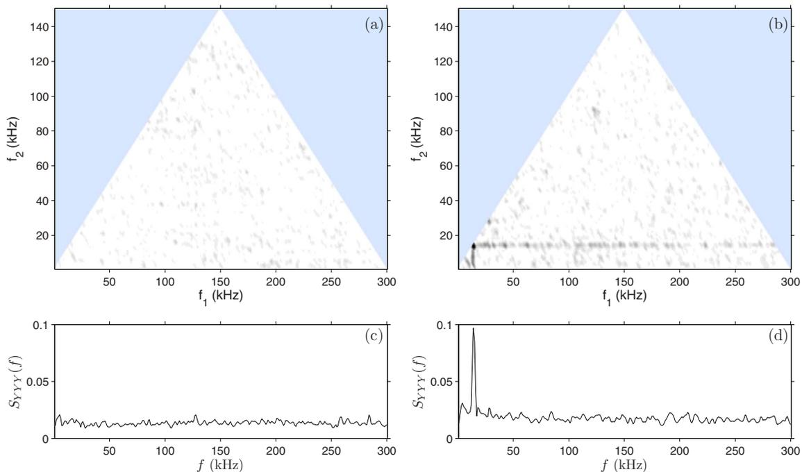
FIG. 6. (Color online) Bicoherence spectrum of electrostatic oscillations ( $b_{\phi_i\phi_j}^2$ ) obtained from numerical integration of Eqs. (10)–(12) with (a)  $A=0.35$ ,  $B=0$ ; (b)  $A=0.35$ ,  $B=0.03$ . (c) and (d) are plots of the summed bicoherence corresponding to (a) and (b), respectively.
