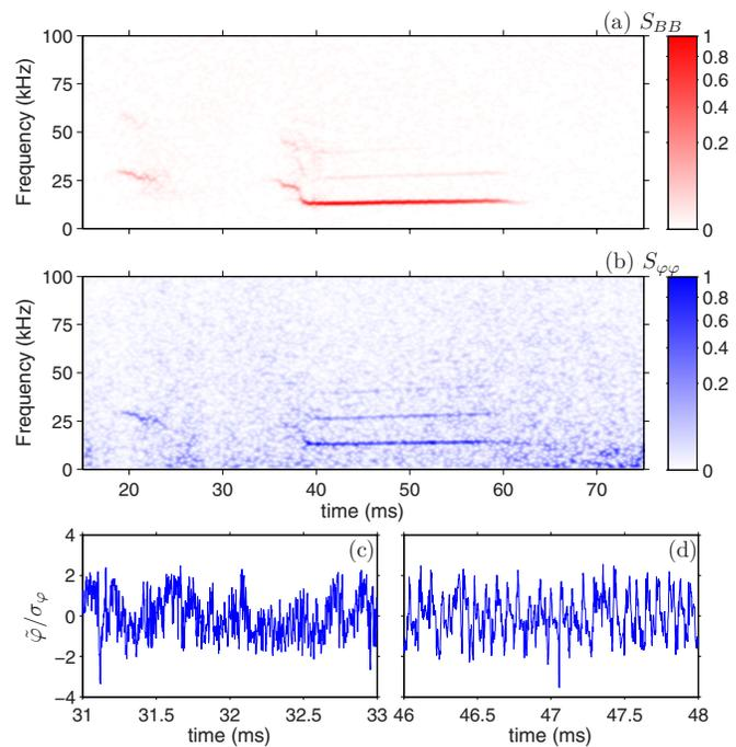
FIG. 2. (Color online) Fourier power spectral density (arbitrary units) for (a) Mirnov oscillations and (b) electrostatic potential at  $r_s/a=0.97$  during the discharge of Fig. 1. Fluctuating electrostatic potential (c) before and (d) during the period with high MHD activity.
