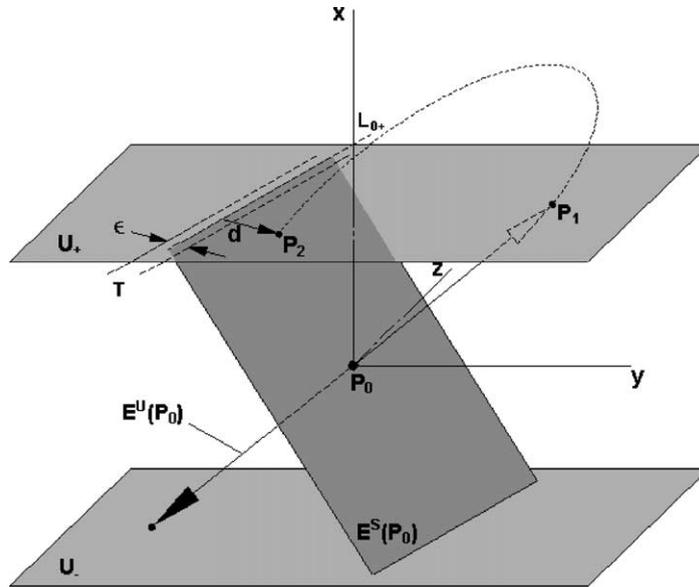
Fig. 3. Representation of the points  $P_1$  and  $P_2$ , that are formed by  $W^U(P_0) \cap U_+$ . We represent the distance between  $L_{0+}$  and  $P_2$  by  $d$ .  $T$  represents a strip of width  $\epsilon$  centered at the line  $L_{0+}$ . A necessary condition for the existence of homoclinic orbits is that  $d = 0$ .
