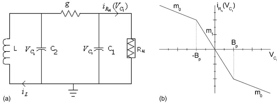
Fig. 1. (a) Schematic diagram of the double-scroll circuit.  $V_{C_1}$  and  $V_{C_2}$  are the potential across capacitors  $C_1$  and  $C_2$ , respectively, and  $i_L$  is the current across the inductor  $L$ . (b) Characteristic curve of the nonlinear resistance  $R_N$ , showing the current  $i_{R_N}$  across  $R_N$ , with respect to  $V_{C_1}$ .
