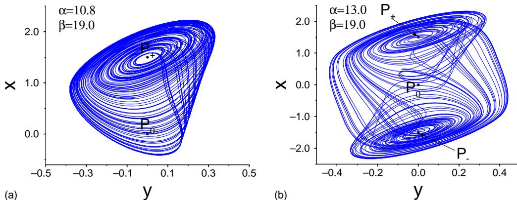
Fig. 10. Two chaotic attractors of the double-scroll system: (a) the Rössler-type attractor for the parameters  $\alpha = 10.8$  and  $\beta = 19.0$ ; (b) the double-scroll attractor for  $\alpha = 13.0$  and  $\beta = 19.0$ .
