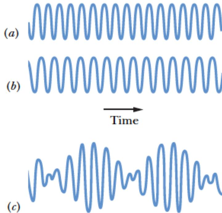
**Fig. 17-17** (a, b) The pressure variation  $\Delta p$  of two sound waves as they would be detected separately. The frequencies of the waves are nearly equal. (c) The resultant pressure variation if the two waves are detected simultaneously.
