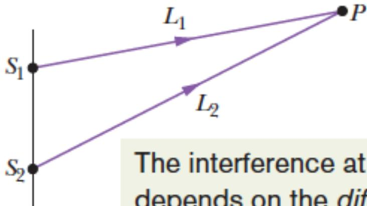
The interference at  $P$  depends on the *difference* in the path lengths to reach  $P$ .
