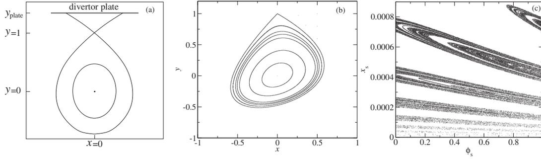
**Fig. 8.** (a) Schematic view of a divertor equilibrium configuration. (b) Phase portrait and (c) magnetic footprint for the simple divertor map with  $k = 0.6$ .
