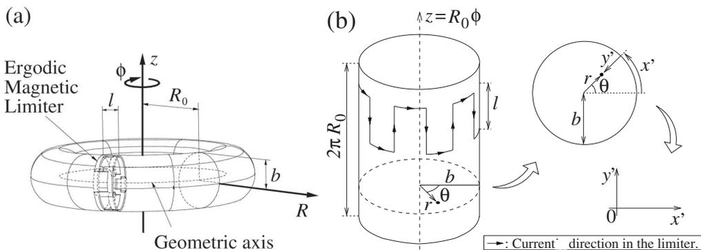
**Fig. 1.** Schematic view of (a) the tokamak toroidal chamber and the ergodic limiter configuration; (b) the periodic cylinder approximation and the rectangular coordinates used to describe field lines.
