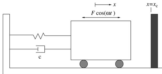
Fig. 1. Model of an impact oscillator.
