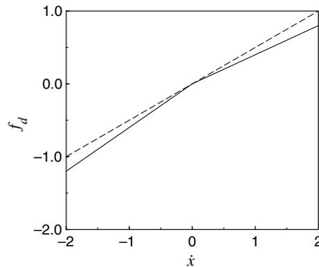
Fig. 6. Damping force  $f_d = c\dot{x} - k|\dot{x}|$ ; for  $k = 0$  uncontrollable damper (dashed line) and for  $k = 0.1$  controllable damper (solid line).
