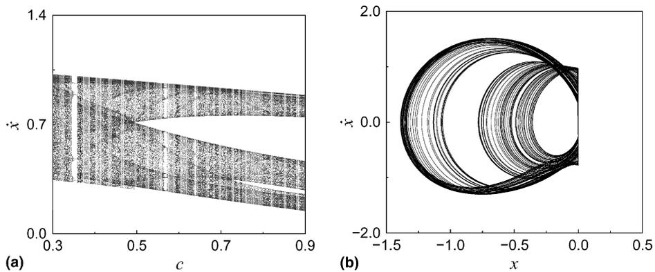
Fig. 2. (a) Bifurcation diagram of the velocity,  $\dot{x}$ , just before the impact as a function of the damping parameter  $c$ ; (b) the phase portrait of the chaotic behavior for  $c = 0.5$ .
