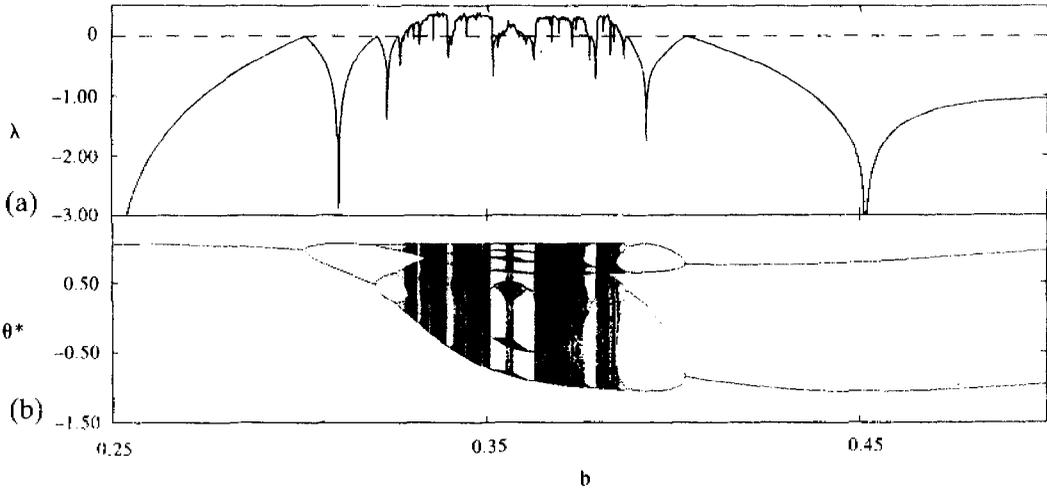
Fig. 6. Lyapunov exponents and bifurcation diagram fixing  $a = 0.57$  and varying the control parameter  $b$ .
