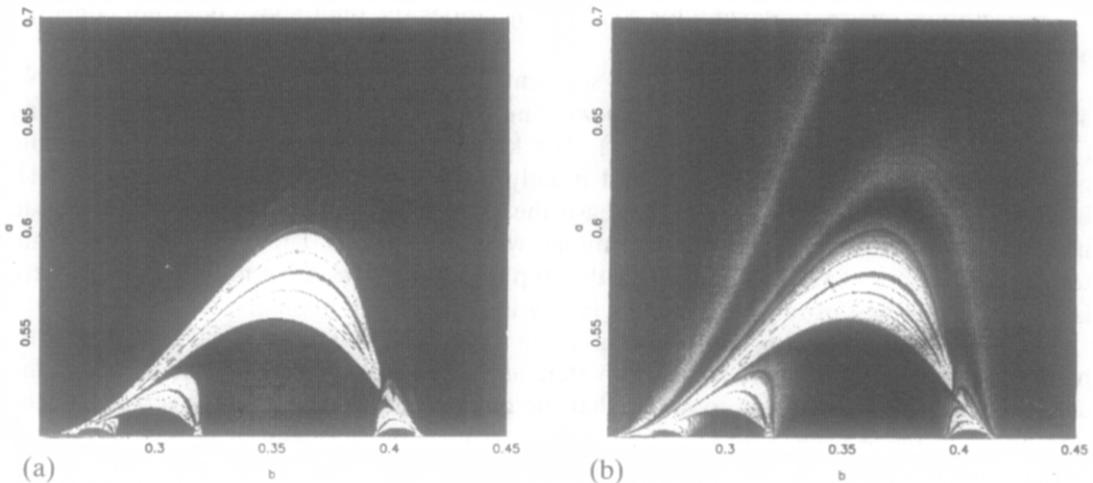
Fig. 2. (a) Isoperiodic diagram around the chaotic region with white points at aperiodic orbits; and (b) Lyapunov exponents with light points for  $\lambda > 0$  and dark points for  $\lambda < 0$ .
