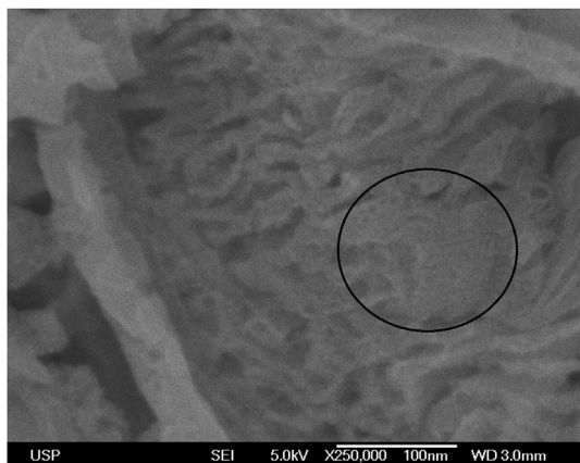
Fig. 11. TEM image of the ZrCe-2 sample with slit like pores and circular pores (circle).
