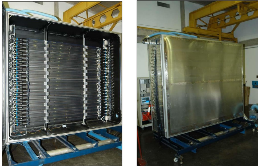
Figure 1: The n-Wall detector system of LAFN with the door open (left) and closed (right).
