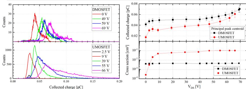
Collected charge spectra of alpha-induced SEEs in the DMOSFET (top) and the UMOFET (bottom) for several  $V_{DD}$ . The charge spectra were normalized to the same fluence.
