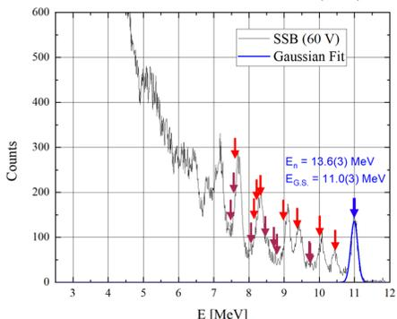
Energy spectrum produced by the interaction of fast neutrons with a fully-depleted SSB detector. The excited levels of <sup>25</sup>Mg (red) and <sup>28</sup>Al (wine) are shown.
