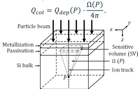
Principle of the diffusion model of Wrobel et al. [6].
