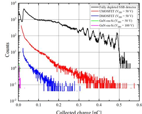
Normalized collected charge spectrum from the interaction of 13.6(3) MeV neutrons with a fully depleted SSB and the power transistors.
