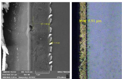
UMOFET parameters were extracted from Scanning Electron Microscopy (SEM) and Optical Microscopy (OM).
