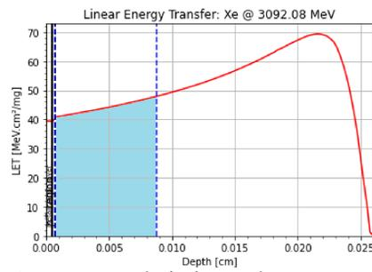
Linear Energy Transfer (LET) curve of 3 GeV Xe on a FET structure. Calculated using SRIM code.
