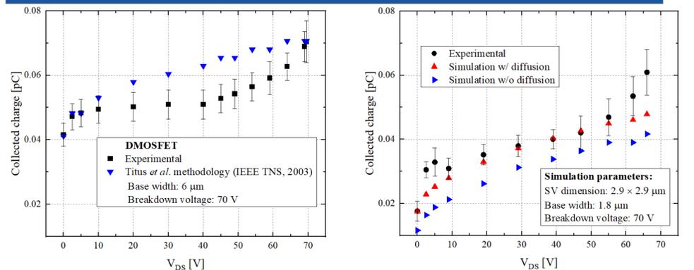
Experimental and calculated collected charge in the DMOSFET induced by 4.8 MeV alpha-particles. Calculations based on model presented by Titus *et al.* (IEEE TNS, 2003).
