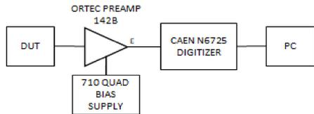
Electronic acquisition system diagram for particle-induced charge spectroscopy in transistors.
