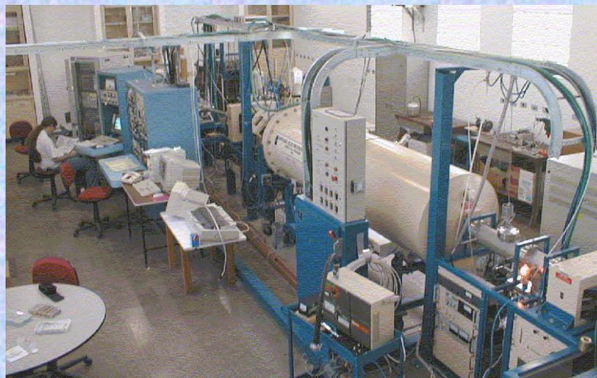
**Multi use vacuum chamber for RBS, PIXE, channeling and ERDA analysis with optional external beam. 5DF goniometer computer based data acquisition and control system.**
