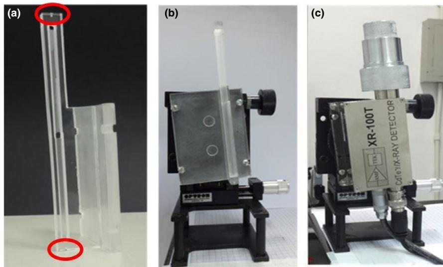
FIG. 2. (a) PMMA alignment device with circles representing the position of the tungsten spheres; (b) the alignment device positioned on the positioning system and (c) the portable CdTe spectrometry system positioned on the positioning system. [Color figure can be viewed at [wileyonlinelibrary.com](http://wileyonlinelibrary.com)]
