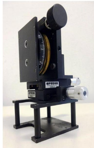
FIG. 1. Positioning system manufactured from the mechanical adaptation of commercial positioners (Optron Ltda, Campinas, Brazil). [Color figure can be viewed at [wileyonlinelibrary.com](http://wileyonlinelibrary.com)]
