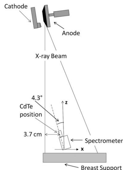
FIG. 6. Position of the aligned spectrometer according to an adopted reference system.
