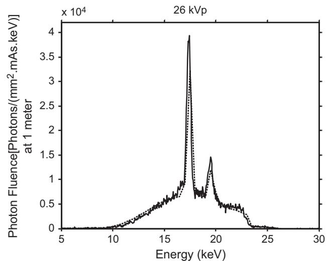
FIG. 8. Experimental (solid line) and computer-generated x-ray spectrum (dashed line) using the MASMIP model: 26 kV (Mo/Rh) spectrum generated by the Selenia equipment.
