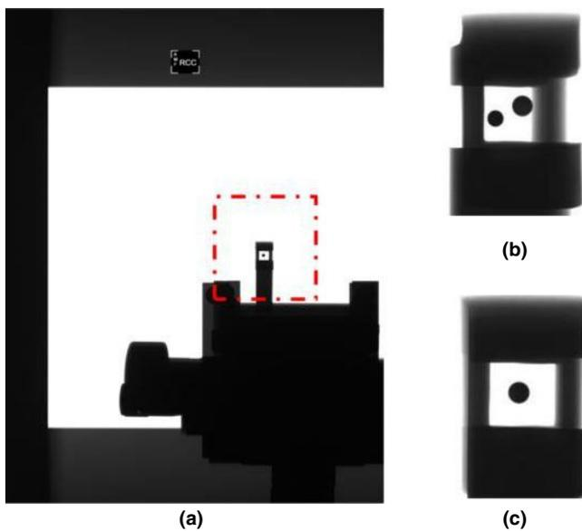
FIG. 4. (a) Radiographic image of the alignment system on the breast support obtained using a 15 cm × 15 cm mammographic radiation field. The dashed box highlights the location of tungsten spheres; Details of the image emphasizing the region of the tungsten spheres when (b) the device is not aligned and (c) the device is aligned. [Color figure can be viewed at [wileyonlinelibrary.com](http://wileyonlinelibrary.com)]
