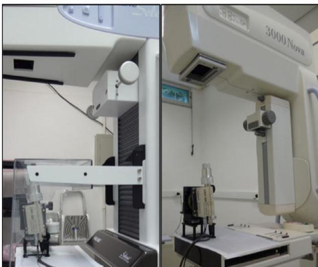
FIG. 5. Positioning of a spectrometer in the two mammography systems used in this study: Selenia (left) and Mammomat 3000 Nova (right). [Color figure can be viewed at [wileyonlinelibrary.com](http://wileyonlinelibrary.com)]
