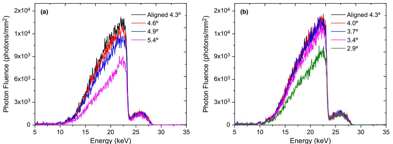
FIG. 10. A comparison of the 28 kV photon fluence spectra measured using W/Rh combination with the spectrometer at different inclinations for angles larger [Fig. 10(a)] and angles smaller [Fig. 10(b)] than the spectrometer angle in the position of alignment (4.3°). [Color figure can be viewed at wileyonlinelibrary.com]
