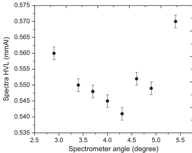
FIG. 11. HVL values derived from the x-ray spectra measured with the spectrometer positioned at different angles.
