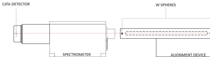
FIG. 3. Cross section of the basic mechanical structure of the spectrometer (based on Amptek Inc.) and alignment device. [Color figure can be viewed at [wileyonlinelibrary.com](http://wileyonlinelibrary.com)]
