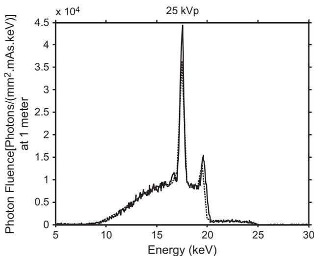
FIG. 7. Experimental (solid line) and computer-generated x-ray spectrum (dashed line) using the MASMIP model: 25 kV (Mo/Mo) spectrum generated by the Selenia equipment.
