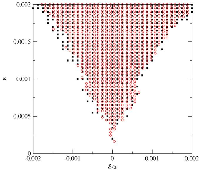
Fig. 6. Empty circles show parameters for which PS exists, detected by Eq. (6), and filled squares represent parameters for which a length-1 PS-set appears simultaneously with a length-2 PS-set with disjoint minimal sets. The horizontal axis represents parameter mismatch and the vertical axis the coupling amplitude.
