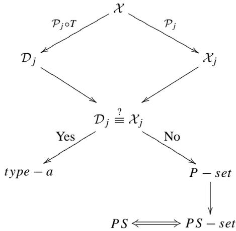
Starting from the chaotic attractor  $\mathcal{X}$ , the set  $\mathcal{D}$  is constructed from the conditional Poincaré map represented by  $T$ ; we project  $\mathcal{D}$  and  $\mathcal{X}$  into the subspace  $\mathcal{P}_j$ , obtaining the sets  $\mathcal{D}_j$  and  $\mathcal{X}_j$ , respectively.
