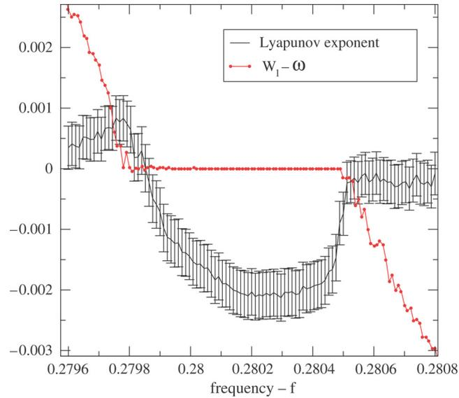
Fig. 4. The Lyapunov exponent (and the error bars) associated with PS in black, and the quantity  $\langle W_1 \rangle - \omega$  in gray, for a fixed amplitude of  $V = 0.0015$  and a varying frequency.
