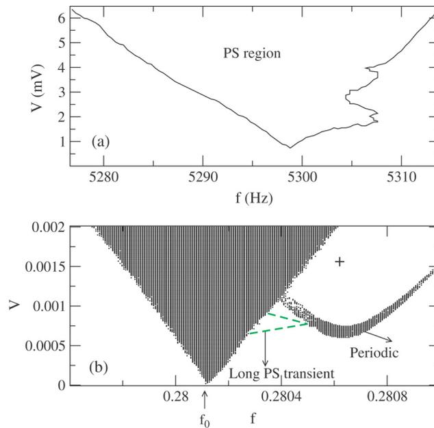
Fig. 2. (a) Experimental PS parameter space. (b) Simulated PS parameter space. Black points represent parameters for which Eq. (6) is satisfied for 120,000 crossings of the trajectory at  $X_2 = 0$ . In both figures, the horizontal axis represents the forcing frequency  $f$  and the vertical axis its amplitude  $V$ . Variables in (b) are dimensionless and  $f_0$  is the main frequency of the non-forced circuit.
