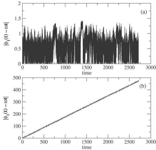
Fig. 1. (a) Phase difference is always smaller than  $2\pi$ , so PS exists between the circuit and the forcing for  $f = 0.2801$  and  $V = 0.0015$ . (b) PS is not present and the phase difference grows bigger than  $2\pi$ .
