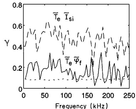
FIG. 8. Coherence at  $r/a=0.92$  of  $\tilde{T}_e$  with  $\tilde{I}_{Si}$  and  $\tilde{\varphi}_f$  (dashed and full curves respectively). Straight line denotes statistical uncertainty.
