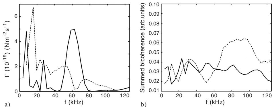
Fig. 5. Superposition of a) the particle transport spectra and b) of filtered summed cross-bicoherence between potential and ion saturation current fluctuations, without (—) or with (---) DC biasing, for time intervals of 1.02 ms at  $r/a = 1.17$ .
