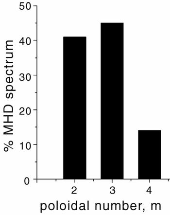
Fig. 2. MHD spectrum of Mirnov oscillations
