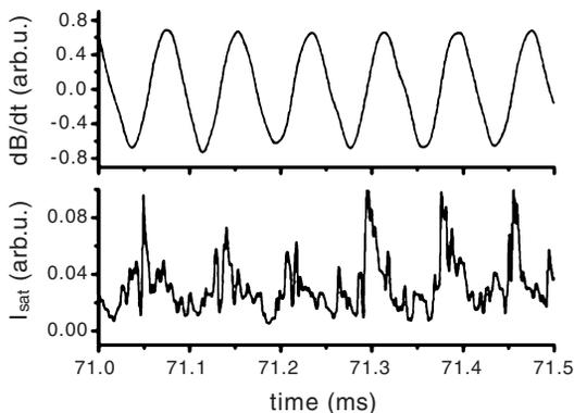
Fig. 1. Oscillations on the Mirnov coil signal and fluctuations of the ion saturation current, for a chosen time interval.
