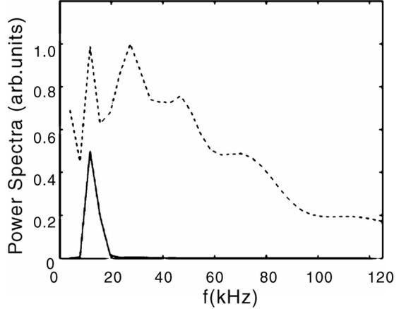
Fig. 3. Superposition of the spectra of Mirnov oscillations (—) and fluctuations of potential (---) at  $r/a = 1.17$ .
