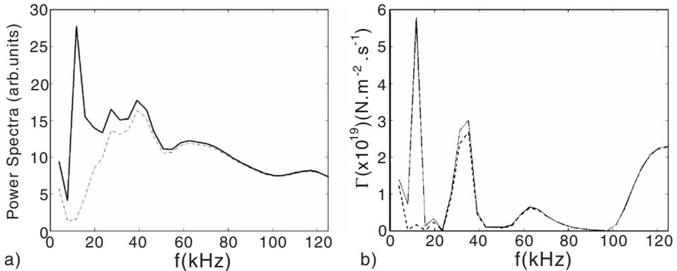
Fig. 4. Superposition of a) the potential fluctuation spectrum and b) the particle transport spectrum (—), and the respective filtered spectra without the frequencies corresponding to Mirnov oscillations (---), for a time interval of 1.02 ms at  $r/a = 1.17$ .
