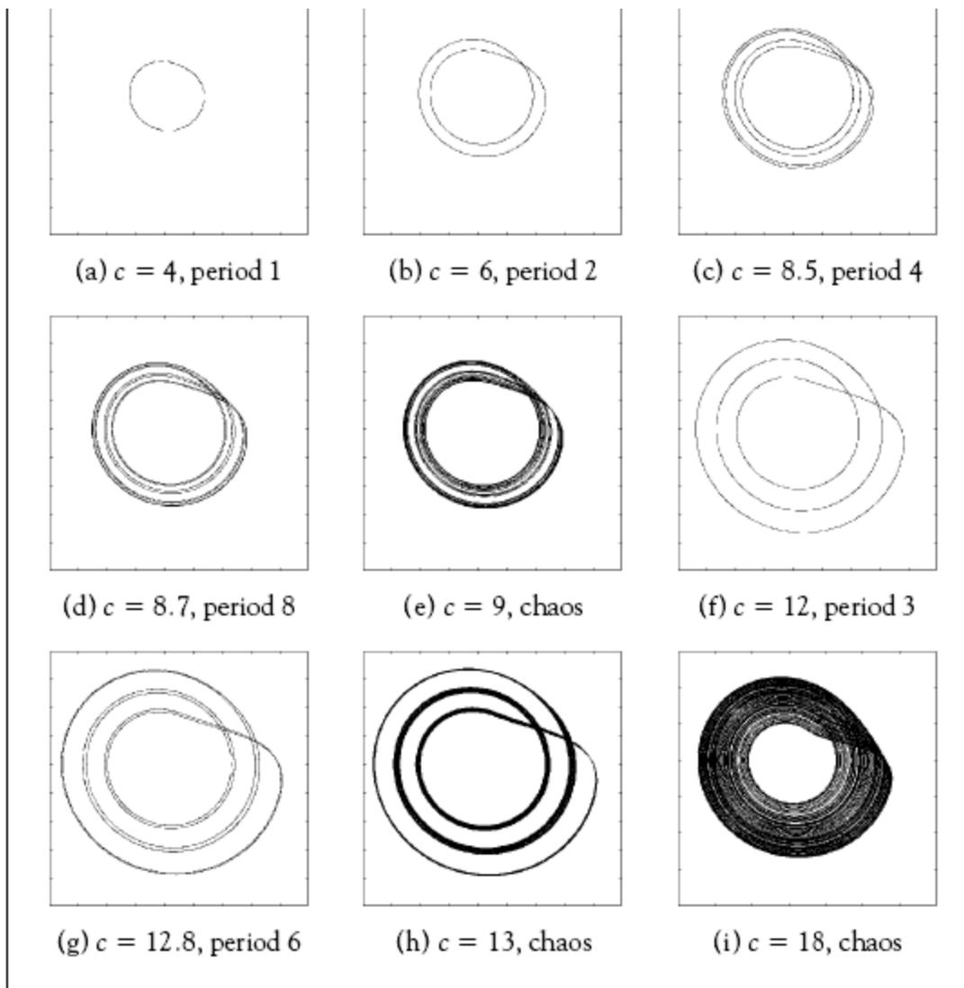
**Figure 9.7** Attractors of the Rössler system as  $c$  is varied.
