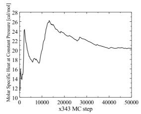
the molar specific heat at constant pressure,  $c_p(cal/mol)$  is shown as illustration of result obtained in a simulation of one furfural and 342 water molecules in the NPT ensemble.
