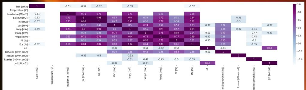
Figure 4: Correlation matrix of sample #3908 after removing the highly doped GaAs cap layer in the optical area of the device
