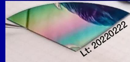
Ga<sub>2</sub>O<sub>3</sub> film deposited on Si(100), with 500 eV ion beam energy
